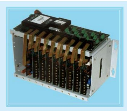
Converters of signalling protocols are stand-alone network modules, which provide interworking of different signalling systems in analog and combined analog/digital telephone networks of the Russian Federation and CIC.
