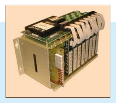
For connection to the converter 3-wire local trunks incoming and outgoing from ATE and 4-wire terminals E&M from a rural ATE are used, and ones are used in both-way mode.
