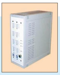
The converter is designed on the base of micro-PC. Cards are made in geometrical sizes of micro-PC (122x112 mm), ones use 62-pin connector, geometrically compatible with ISA connector of a system bus of micro-PC.
