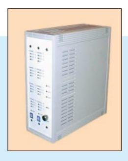
The converter is designed on the base of mini-PC. Cards are made in geometrical sizes of micro-PC (122x112 mm), ones use 62-pin connector, geometrically compatible with ISA connector of a system bus of micro-PC.
